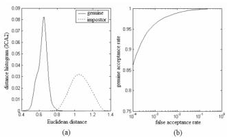
Fig. 10. Verification results of the  $ICA_2$ -based method: a) Genuine and impostor distance histograms; b) ROC curve.
