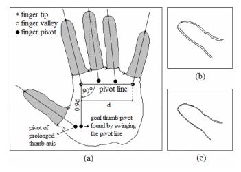
Fig. 5. a) Fingers extracted by a sickle sweep, finger axes, finger pivots and definition of hand pivotal axis; b) Thumbs of the same person overlapped after rotation; c) Thumbs of the same person overlapped after rotation and pivotal translation.
