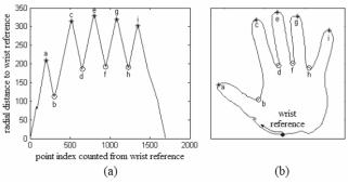
Fig. 3. a) Radial distance function for finger extraction; b) A hand contour with marked extremities.
