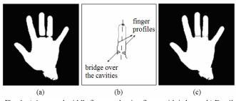
Fig. 4. a) A severed middle finger and a ring finger with isthmus; b) Detail of finger isthmus; c) Hand image after ring artifact removal.
